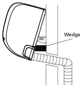
3. Connect drain hose and refrigerant piping (refer to **Refrigerant Piping Connection** section of this manual for instructions).
