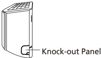
3. If existing connective piping is already embedded in the wall, proceed directly to the **Connect Drain Hose** step. If there is no embedded piping, connect the indoor unit's refrigerant piping to the connective piping that will join the indoor and outdoor units. Refer to the **Refrigerant Piping Connection** section of this manual for detailed instructions.
