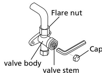
12. Using hexagonal wrench, fully open both the high pressure and low pressure valves.
